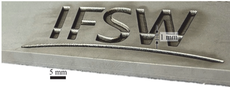
Figure 4.6 Photograph of the logo of the institute micromachined on a stainless steel sample with a resulting depth of 1 mm. Process parameters: \lambda_L = 1030 nm, P = 1010 W, f_B = 500 kHz, E_B = 2020 \mu J, N_{ppb} = 5 , \phi_0 = 0.74 J/cm 2 , d = 372 \mu m, v_x = 24 m/s, p_y = 40 \mu m, m = 350 .
