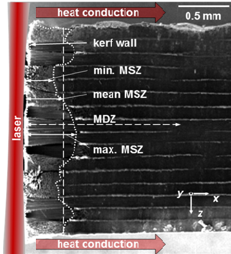
Fig. 1: Scanning electron microscope (SEM) picture of a cross section of the material. The arrows with solid lines show the measured minimum, maximum, and mean MSZ in layers with different fiber orientations. The dashed arrow symbolizes the maximum calculated MDZ.
