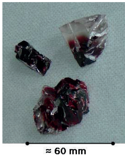
Figure 3.9: Example of as grown Yb:Lu 2 O 3 pieces.
