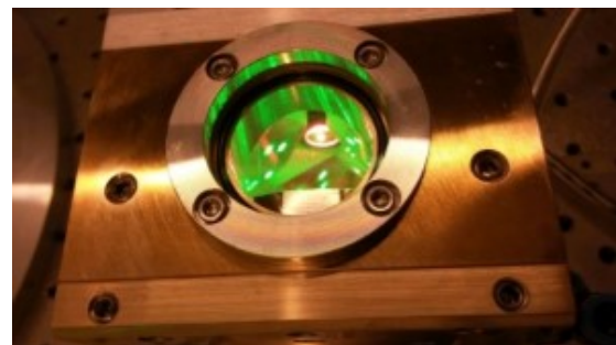
Fig. 2: 48-passes thin-disk pumping module (B1-48).
