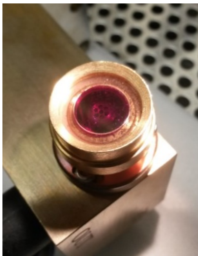
Fig. 1: Thin-disk Ti:Sa laser crystal mounted on a diamond heat sink
