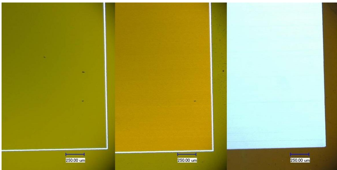
Fig1: left SiN-coated Pt surface; centre only selectively ablated SiN, right additional Pt cut
