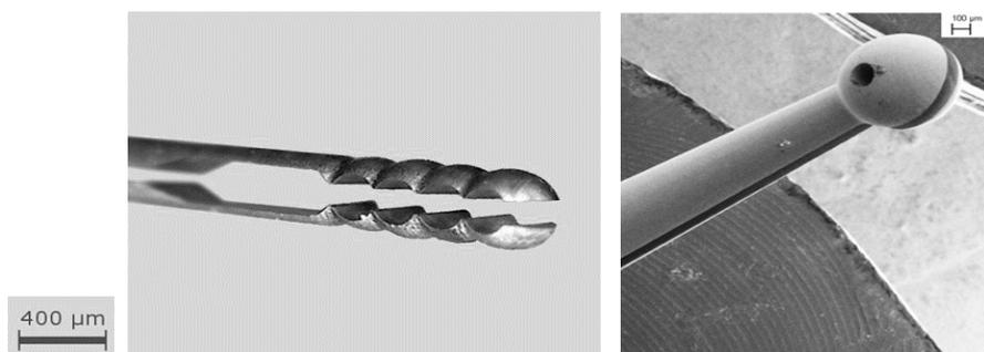
Stainless steel micro tweezers for medical industry, laser turned, cut / drilled with GL.trepan
