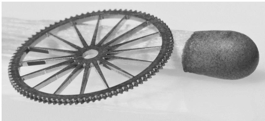
Brass micro gear wheel for watches cut with sub-picosecond laser and GL.trepan; feed rates from 10 - 200mm/min depending on material and material thickness
