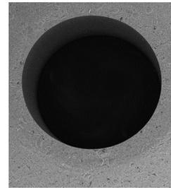
Cylindrical hole in 300µm steel for fuel injection applications, drill time < 1.5s
