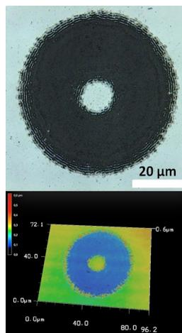
Figure showing the femtosecond ablation on a 100 nm thick platinum layer using radial polarization. Due to the polarization type, SLV were able to ablate about 15% more platinum as with linear polarization at the same pulse energy.
