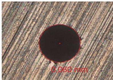
Ø 60µm in 0.5mm heavy metal for textile industry; drill time 3s with 515nm
