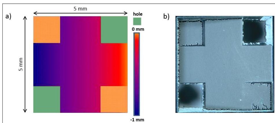
**Figure 2: Profile of model geometry (a) and structure machined into silicon wafer using parameters of Table 2 (b).**
