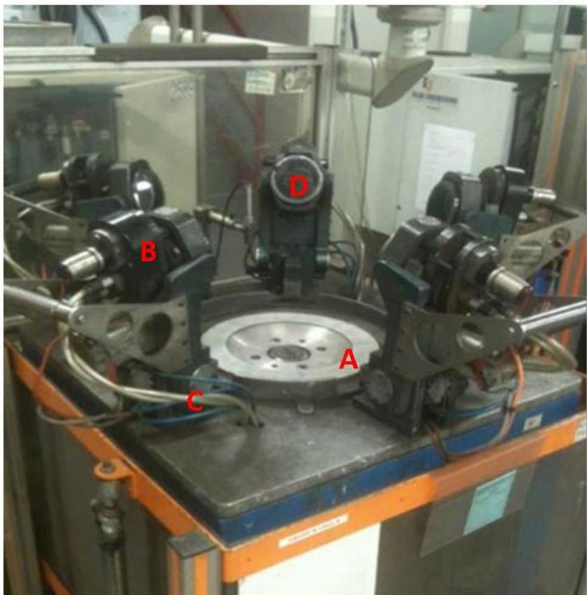
Figure 8: Picture of a polishing machine in Element Six
