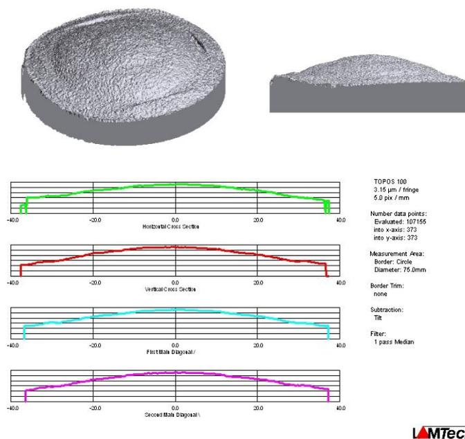
**Figure 13: Flatness measurement of domed surface of pre-polished Syndite disc using interferometric measurement device**
