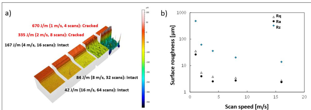
**Figure 6: Measurement data of structures machined with the high-power USP laser system available at IFSW; a) surface roughness measured by white light interferometry on structures created at different feed velocities; b) corresponding surface roughness values**
