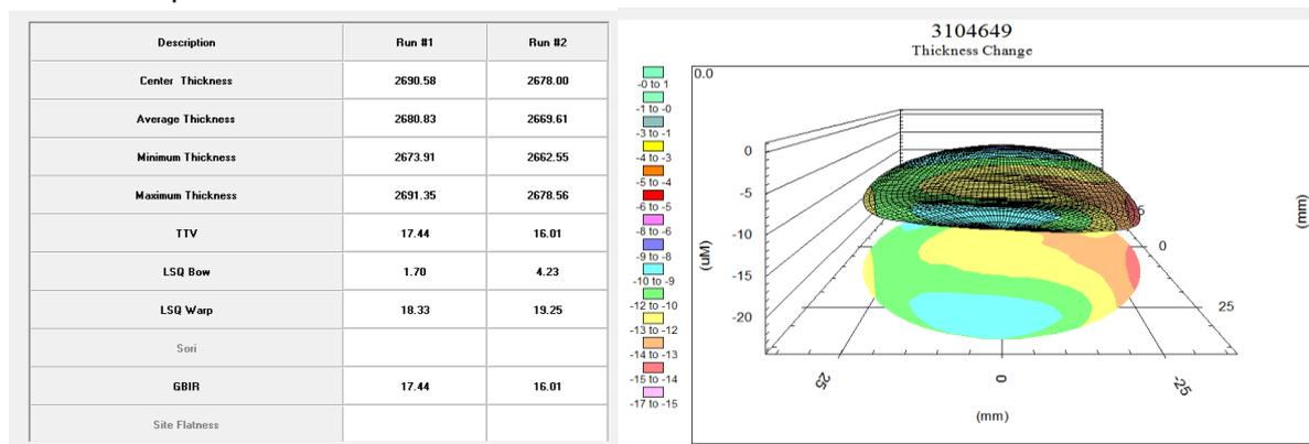
**Figure 12: Results from Proforma measurement (thickness variation = 11.22  $\mu\text{m}$ , after 6 hours of mechanical polishing)**
