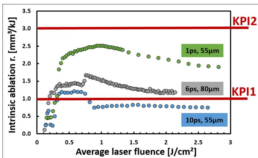
**Figure 4: Intrinsic ablation rate of silicon ablation with different laser sources as a function of laser fluence**
