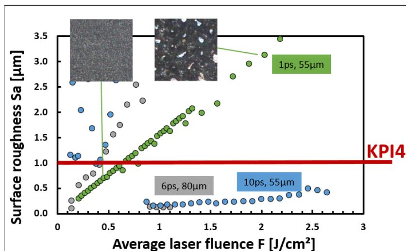
**Figure 5: Roughness of ablated silicon surfaces as a function of laser fluence for different laser pulse durations.**
