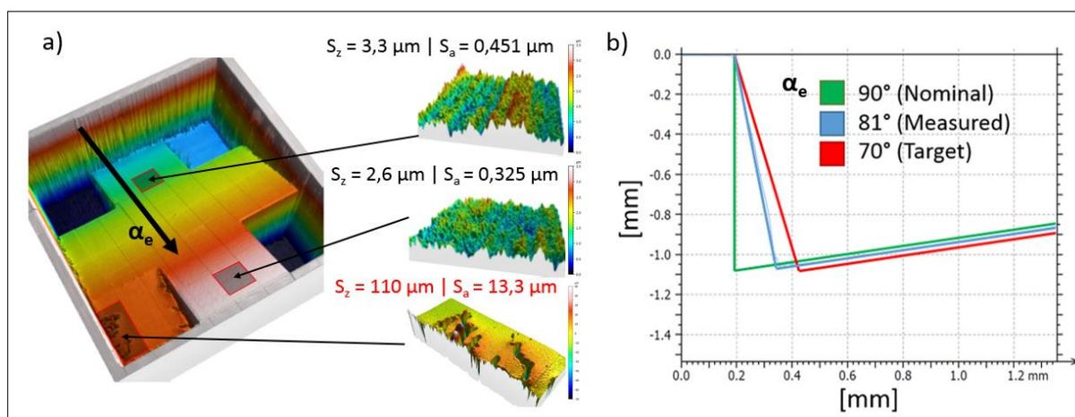
**Figure 3: White light interferometry measurements of the ablated structure shown in Figure 2; a) model geometry and roughness values; b) edge steepness measurement**
