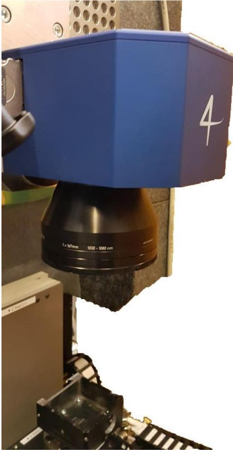
*Figure 5: Qioptiq 167 mm lens with mounting adjustment and corresponding correction file mounted on C4L galvo-housing*
