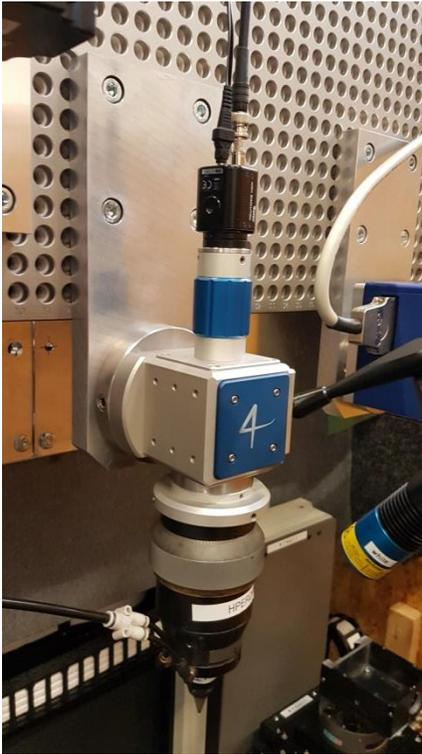
*Figure 9: C4L gas assisted cutting head mounted with assist gas connected*
