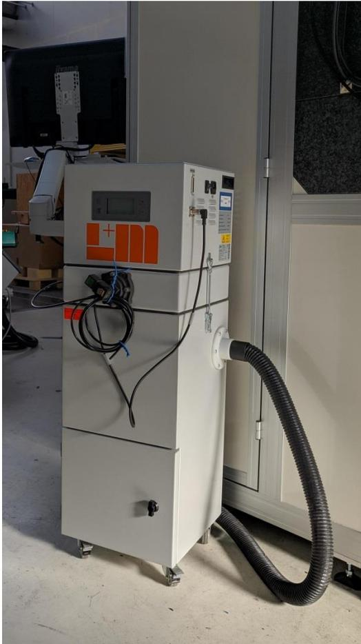
*Figure 7: TBH fume extraction system connected to sample fixation unit*
