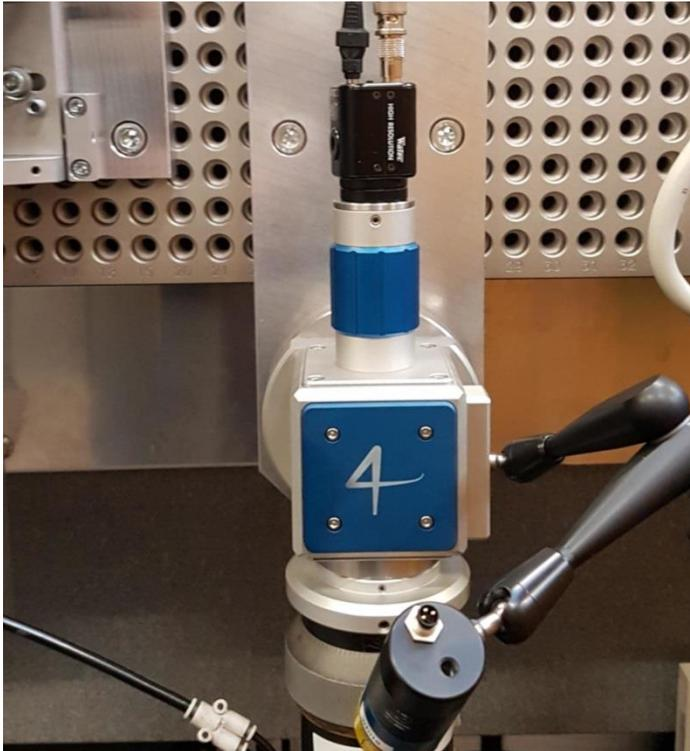
*Figure 6: Watec WAT-902B CCD camera mounted on C4L gas assisted cutting head with corresponding light source and adaptable focal lens*
