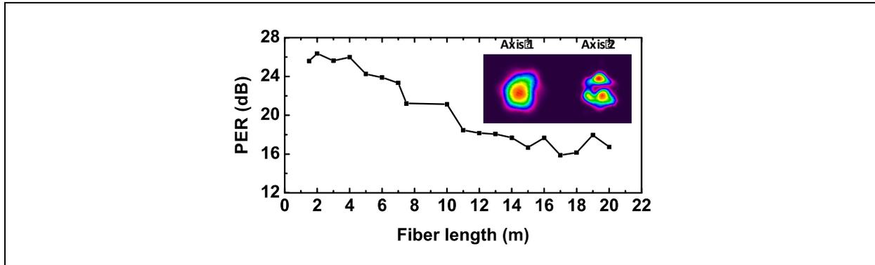
Fig. 4. Linear characterizations of the fiber #1 on the evolution of the PER versus the fiber length.
