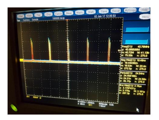
1280 kHz, 3 pulse burst before amplifier
