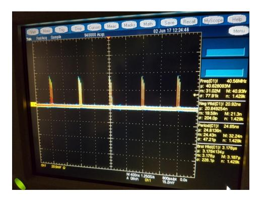
1280 kHz, 3 pulse burst at 500 W output power (power curve is unchanged)
