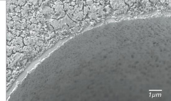
Detailed view of a helically drilled microhole
