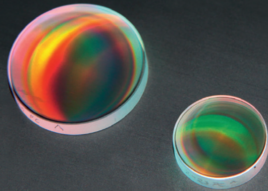
Grating mirrors for pulse compression, with substrate diameters of 38.1 mm and 25 mm
