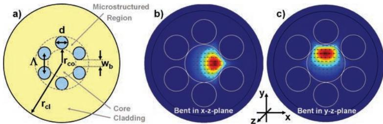
**Figure 5.22:** a) Scheme of a LCF. The intensity distribution of the fundamental mode is deformed and shifted due to a bent in the x-z-plane b) and a bent in the y-z-plane respectively c).
