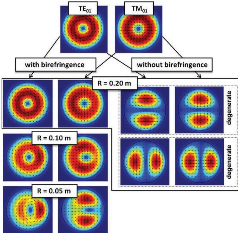
**Figure 7.6:** Calculated intensity distributions of the  $TM_{01}$  and  $TE_{01}$  modes and their modifications if the fiber is bent with a radius  $R$ . In presence of radial-azimuthal birefringence (here max.  $5 \cdot 10^{-4}$  at the core-cladding interface) the modes are maintained which is not the case without birefringence.
