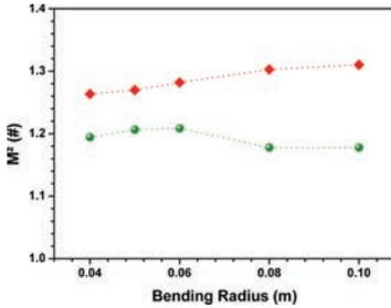
**Figure 6.10:** The  $M^2$ -factors determined in the two main axes after the 7-core fiber are largely independent of the bending radius  $R$ .
