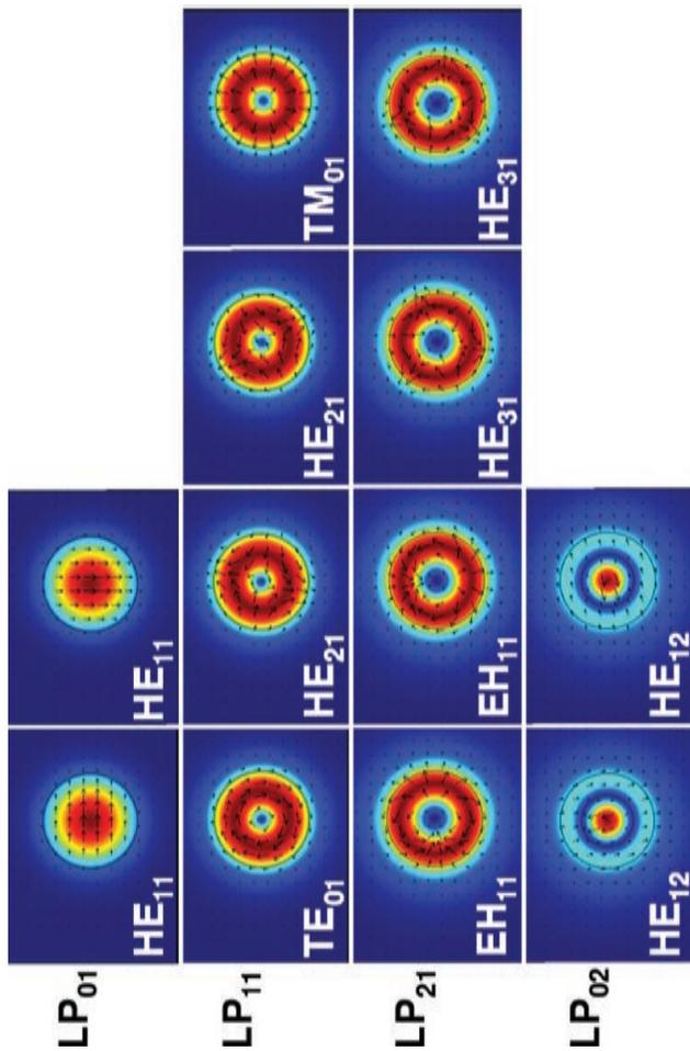
**Figure 2.2:** Calculated mode structure of a step index fiber ( $r_{co} = 30 \mu\text{m}$ ,  $\text{NA} = 0.06$ ). The color distribution corresponds to the intensity of the electric field and the arrows correspond to the polarization of the electrical field. The linearly polarized LP modes can be generated from superpositions of the exact solutions (TE, TM, HE, EH).
