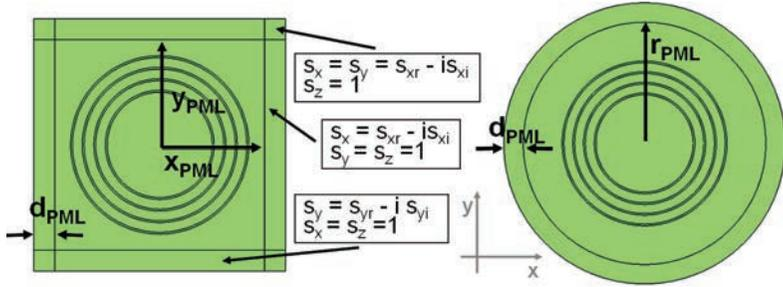
**Figure 3.2:** Scheme of a rectangular and a circular PML with thickness  $d_{\text{PML}}$  surrounding a Bragg fiber. Different damping constants ( $S_{xi}, S_{xi}$ ) along the Cartesian coordinates can be implemented in the rectangular PML.
