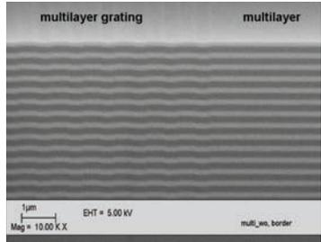
**Figure A.6:** SEM micrography of a multilayer mirror with a multiple-corrugated grating.
