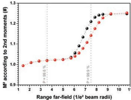
**Figure 5.7:**  $M^2$ -factor calculated for the two main axes. The obtained  $M^2$ -factor depends on the size of the area on which the far-field is calculated and therefore on the power which is cut. Two power levels contained within a certain far-field range are indicated by gray dotted lines.
