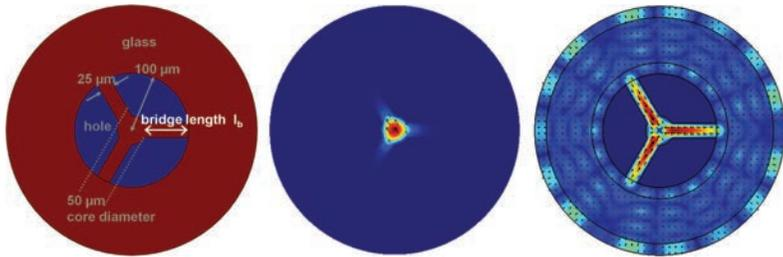
**Figure 5.33:** Scheme of an extended LCF concept. The losses of the fundamental mode can be adjusted by the bridge length  $l_b$ . The geometrical parameters of such an investigated fiber are indicated in gray. The calculated  $LP_{01}$  and  $TM_{01}$  modes corresponding to this parameters are shown.
