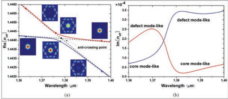
Figure 2.5: Analyses of real parts (a) and imaginary parts (b) of the effective mode indices  $n_{\text{eff}}$  of two modes as a function of the wavelength taken from [24] in case a complete coupling occurs. The insets show the intensity distributions of the coupled modes at selected wavelengths.
