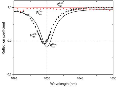
**Figure A.4:** Measured and calculated reflection coefficients of a grating with a period of 930 nm and of a nominal groove depth of 15 nm combined with a standard 29 quarter-wave layer dielectric mirror.
