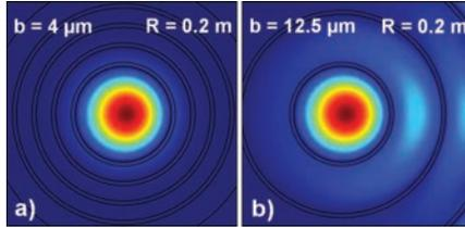
**Figure 5.15:** Calculated electric field distribution of the fundamental mode at a bending radius of  $R = 0.2 \text{ m}$  for two BFs with  $b = 4 \mu\text{m}$  a) and  $b = r_{co} = 12.5 \mu\text{m}$  respectively b).
