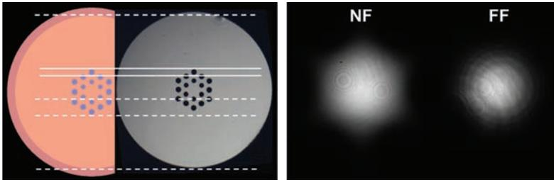
**Figure 5.29:** CLCF18 end face microscope picture, scaled according to the measured outer diameter and compared to the design. White lines are reference guides to the eyes (LHS). Measured NF and FF distribution (RHS).
