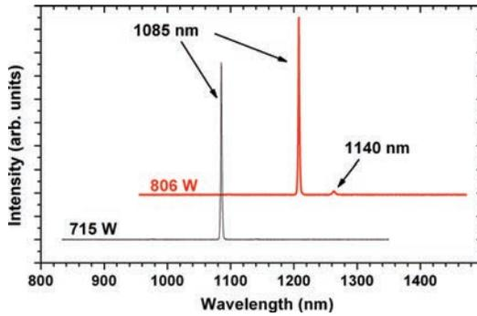
**Figure 6.7:** Spectral intensities after a passive beam delivery fiber ( $r_{co} = 15\mu\text{m}$ ,  $\text{NA} = 0.056$ ) of 100m length. At high output powers the onset of SRS, indicated by an small peak at 1140 nm, is observed.
