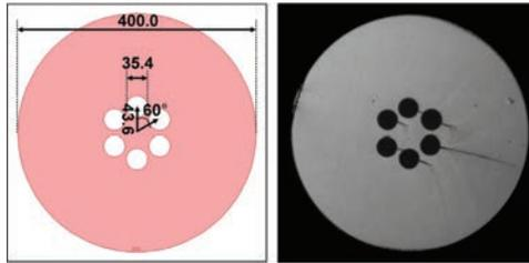
**Figure 5.31:** Design of the fiber (left) and a microscope photograph of the end face of the produced LCF (right). The fiber with a core diameter of  $51.8\ \mu\text{m}$  efficiently guides  $LP_{01}$  and  $LP_{11}$  modes.
