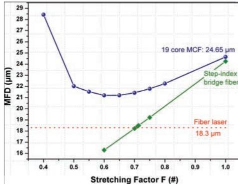
**Figure 5.8:** Calculated MFD of the 19-core fiber for varying geometrical stretching factors  $F$ . A tapered bridge fiber is needed in order to match the MFD of the 19-core fiber to the fiber laser source (red dotted line).
