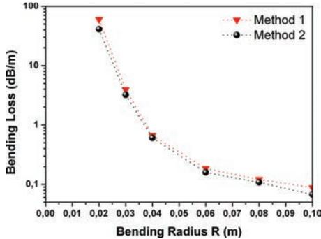
**Figure 4.3:** Results of the bending loss measurements of a low-NA step index fiber with a core diameter of  $30\ \mu\text{m}$ . Bending method 1 (red triangles) results in higher losses than method 2 (black circle) due to a mode mismatch at the points where the straight fiber is abruptly bent with a radius  $R$ .
