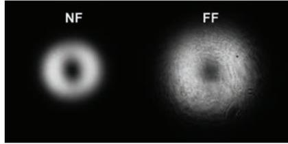
**Figure 7.3:** Near- and far-field intensity distributions after a 10 m long fiber with  $25\ \mu\text{m}$  core diameter and a NA of 0.07 if a radially polarized  $\text{TM}_{01}$  mode was coupled to the fiber.
