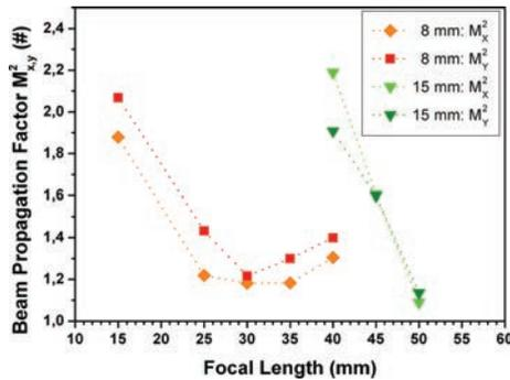
**Figure 6.1:** Beam propagation factor  $M^2$  measured after the LMA-GDF-30/400. For each measurement different optics were used to couple the laser beam into the fiber. Two different lens combinations with  $f = 15$  mm (triangles) and  $f = 8$  mm (rectangles) were used to collimate the free space beam resulting in beam diameters of about 1.5 mm and 2.9 mm respectively before the beam was focused into the fiber with different lenses with  $f = 15..50$  mm.
