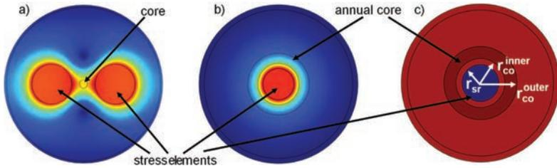
**Figure 7.5:** Calculated stress distribution (Tresca stress) of a Panda-type fiber a) and a fiber with a ring-shaped core and a central stress element b). A scheme of the structure with the central stress element is shown in c).
