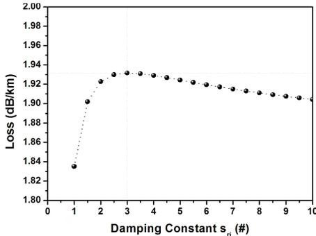
**Figure 3.1:** Effect of the variation of the damping constant  $s_{ri}$  on the calculated losses for a  $10\ \mu\text{m}$  thick perfectly matched layer.
