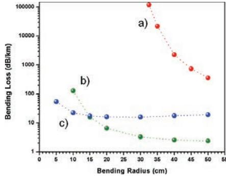
**Figure 5.14:** Simulated bending losses of three BF which only differ in the thickness  $b$  of the low-index layers (a) red:  $b = r_{co} = 12.5\mu\text{m}$ , b) green:  $b = 8.25\mu\text{m}$ , c) blue:  $b = 4\mu\text{m}$ ,  $r_{co} = 25\mu\text{m}$ ,  $n_{co} = n_b = 1.45$ ,  $n_a = 1.47$ ).
