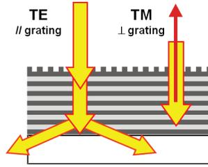
**Figure A.2:** Principle of the microstructured multilayer mirror which introduces a reflectivity difference for TE and TM polarized beams.
