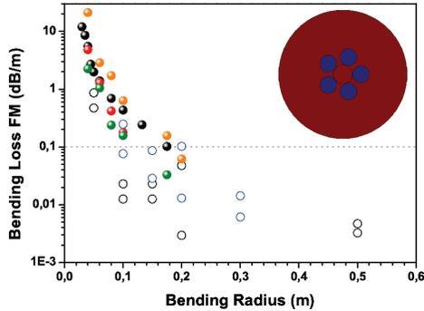
**Figure 5.24:** Different measurements of the bending losses (filled circles) are compared to the simulation results (open circles).
