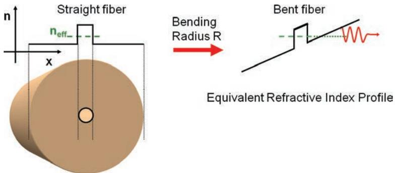
**Figure 3.4:** Principle of the equivalent index model used to simulate bent waveguides in a 2D-environment. The distribution of the refractive index of a straight waveguide is transformed to take into account the curvature.
