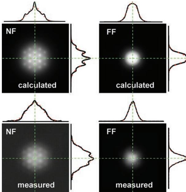
**Figure 5.3:** Calculated and measured intensity distributions of the NF and the FF of the 19-core fiber. Line scans along the two dashed axes are plotted as solid lines and Gaussian fits as dotted lines.
