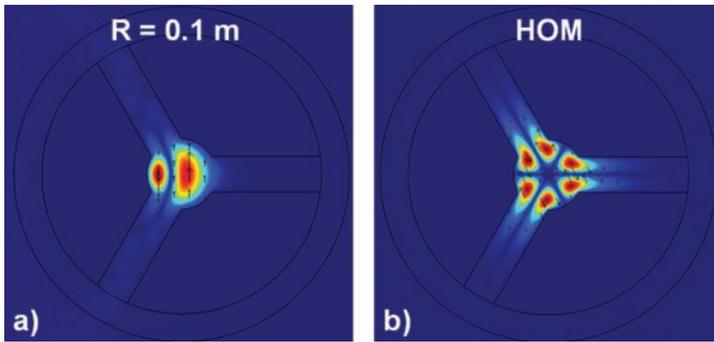
**Figure 5.34:** Lowest-order eigenmodes of the extended LCF concept (with geometrical parameters shown in figure 5.33) if the fiber is bent with  $R = 0.1\text{m}$  a). Because of the symmetry, the structure possesses a weakly core-guided  $LP_{31}$  mode b) but no  $LP_{21}$  mode.
