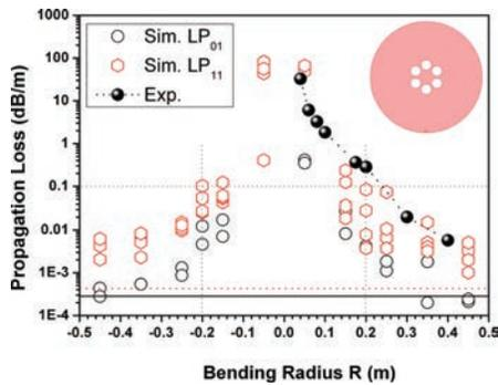
**Figure 5.32:** Bending losses of a LCF suitable to deliver the 2-times polarization degenerate fundamental LP<sub>01</sub> mode and the 4-times degenerate LP<sub>11</sub> mode. The open symbols correspond to the simulated results. Positive R values specify bends in the x-z-plane and negative values specify bends in the y-z-plane. For the measured results, the direction of the bend in reference to the hole structure is unknown and marked only on the positive side (black filled symbols).
