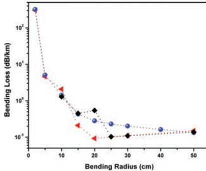
**Figure 3.3:** Calculation of the bending losses of a BF to compare the performance of different PML techniques. The results obtained with the PML according to [50] are indicated by red rectangles, the Comsol Multiphysics 3.3 PML by black diamonds, and results obtained with the PML defined according to [44] are indicated by blue spheres.
