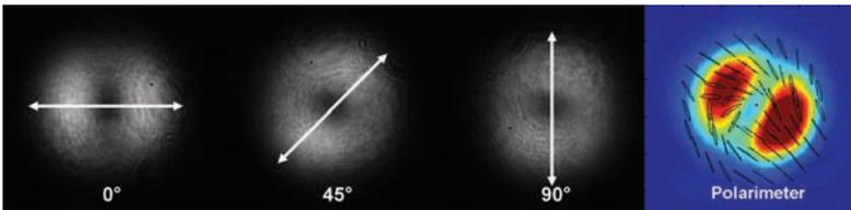
**Figure 7.4:** Distributions of the NF intensity at different analyzer settings are shown together with a false color plot obtained with a polarimeter to measure the local polarization. The measurements were performed after a step index fiber of 10 m length ( $r_{co} = 12.5\ \mu\text{m}$ ,  $\text{NA} = 0.07$ ) to which a radially polarized mode was coupled.
