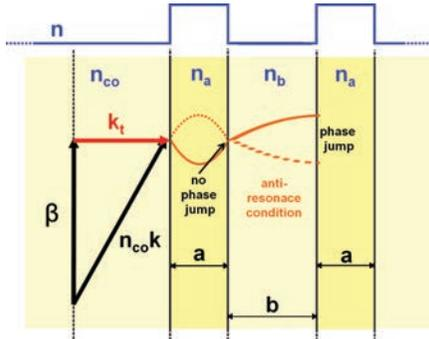
**Figure 5.13:** Propagation constant  $\beta$  in a vector picture. With the transverse component of the wave vector  $k_t$  and an anti-resonance condition the ideal layer thickness  $b$  can be derived.
