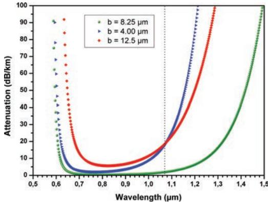
**Figure 5.17:** Comparison of the calculated bandwidth of the three BFs with different low-index layer thicknesses  $b$ .
