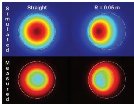
**Figure 6.3:** Bend-induced deformation of the fundamental mode of the LMA-GDF-30/400 if the fiber is bent with  $R = 0.05$  m. The comparison between simulation and experiment shows a good agreement (color schemes are different for the simulation and experimental results).
