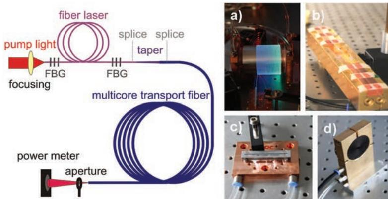
**Figure 5.10:** Scheme of the experimental setup used for high-power fundamental mode delivery. Photographs of the fiber laser a), the 2nd splice b), the water cooled taper c), and aperture d) are shown.
