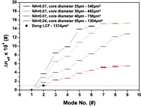
Figure 6.4: Difference of the effective refractive index  $\Delta n_{\text{eff}}$  between the calculated HOMs and the fundamental mode of different step index fibers. In addition, the simulation results for a LCF according to the parameters of [41] are indicated by black pentagons.
