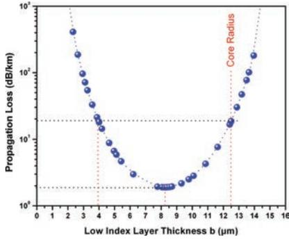
**Figure 5.12:** Calculated propagation losses of a large mode area ( $25\mu\text{m}$  core diameter) BF with 4 high-index layers with varying thickness  $b$  of the low-index layers. The red dotted lines indicate the three values of  $b$  which are used for the following comparison of the bending sensitivity.
