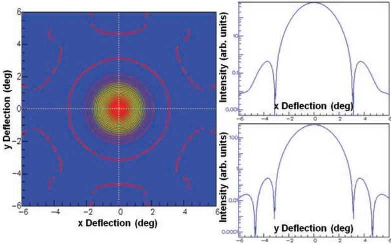
**Figure 5.6:** Intensity distribution of the FF calculated for the supermode of the 19-core fiber showing the diffraction pattern. The red contour lines correspond to equal intensity levels. The two curves on the right show the intensity along the two dotted lines on a logarithmic scale.
