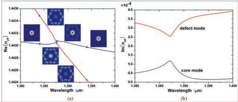
Figure 2.6: Analyses of real parts (a) and imaginary parts (b) of the effective mode indices  $n_{\text{eff}}$  of two modes as a function of the wavelength taken from [24] in case an incomplete coupling occurs. The insets show the intensity distributions of the coupled modes at selected wavelengths.
