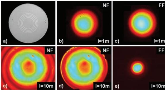
**Figure 5.19:** Photograph of the end face of a BF taken through a microscope a). The four high-index layers are slightly brighter than the undoped fiber parts. Measured near- and far-field patterns after a fiber of  $l = 1$  m length (first row) and a longer fiber of about 10 m length (second row). The high-index rings are visible in c) because some light was captured by index-guiding. These rings were cut with the help of a NF aperture in d).
