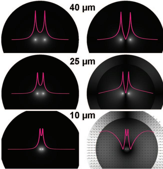
**Figure 5.1:** Symmetric (left) and antisymmetric (right) coupling of 2 SM waveguides (fiber cores) at core-to-core distances of 40, 25 and 10 μm. The optical intensity is displayed in a gray scale picture together with a curve along the cross-section which intersects both cores.
