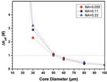
Figure 6.5: Calculated mode spacing  $\Delta n_{\text{eff}}$  of the  $LP_{01}$  and  $LP_{11}$  modes depending on the core diameter for three different NAs.
