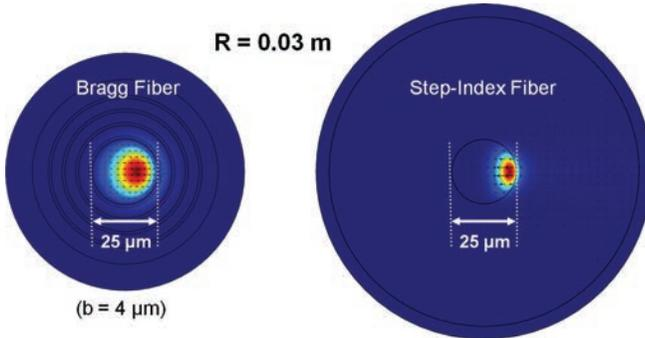
**Figure 5.16:** Comparison of the bend-induced field deformation ( $R = 0.03 \text{ m}$ ) of the FM of a BF with a small layer thickness of  $b = 4 \mu\text{m}$  and a step index fiber ( $\text{NA} = 0.07$ ) with the same core diameter.
