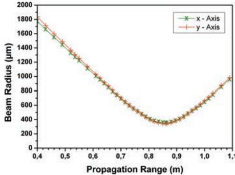
**Figure 5.5:** Measured beam caustic after the 19-core fiber. The measurement in two orthogonal directions (green/red) reveals  $M^2$ -factors of  $M_x^2 \approx M_y^2 \leq 1.03$  and an eccentricity of the beam of 1.03.
