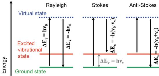
**Figure 2.3:** Photon scattering energy scheme. If the incident (i) and the scattered photon (s) have the same energy, the photon is Rayleigh scattered. If the scattering leads to an excited vibrational state (v), the resulting Stokes-scattered photon has a lower energy. The scattered photon may receive energy from an already excited state which leads to anti-Stokes scattering.
