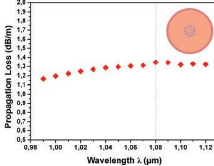
**Figure 5.28:** Wavelength dependence of the resonant mode coupling at a cladding diameter of  $387.58 \mu\text{m}$  of the CLCF18. The graph shows the calculated losses of the  $LP_{11}$  mode at different wavelengths.
